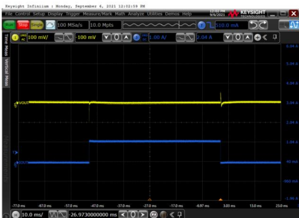
Figure 6. I_{OUT} = 1 mA-1 A TPL910 without C_{FF} during a load transient TPL910 load transient waveform ( C_{FF} = 10 nF )
