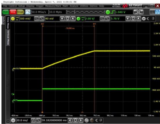
Figure 3. Start-up Waveform (CNR = 100 nF, IOUT = 100 mA)
