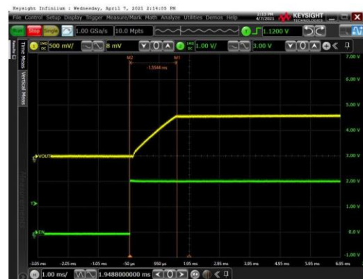
Figure 2. Start-up Waveform ( C_{\text{NR}} = 10 \text{ nF} , I_{\text{OUT}} = 100 \text{ mA} )
