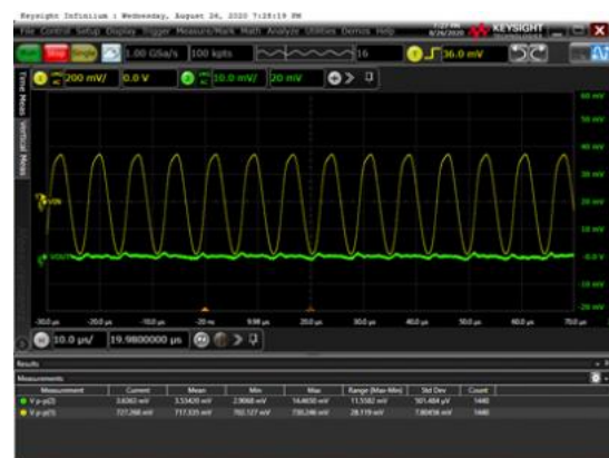
Figure 1. Input and Output Ripples of LDO Measured Using an Oscilloscope
