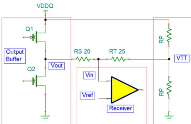
Figure 1. Source Bus Terminal Wiring Diagram
