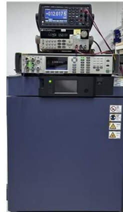
Figure 2-1 TPR70ULTC Temperature Coefficient Test Environment
