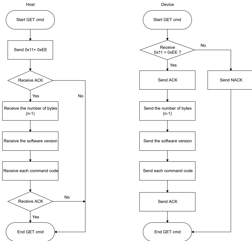
Figure 3-3 USART Bootloader GET Flow Chart
