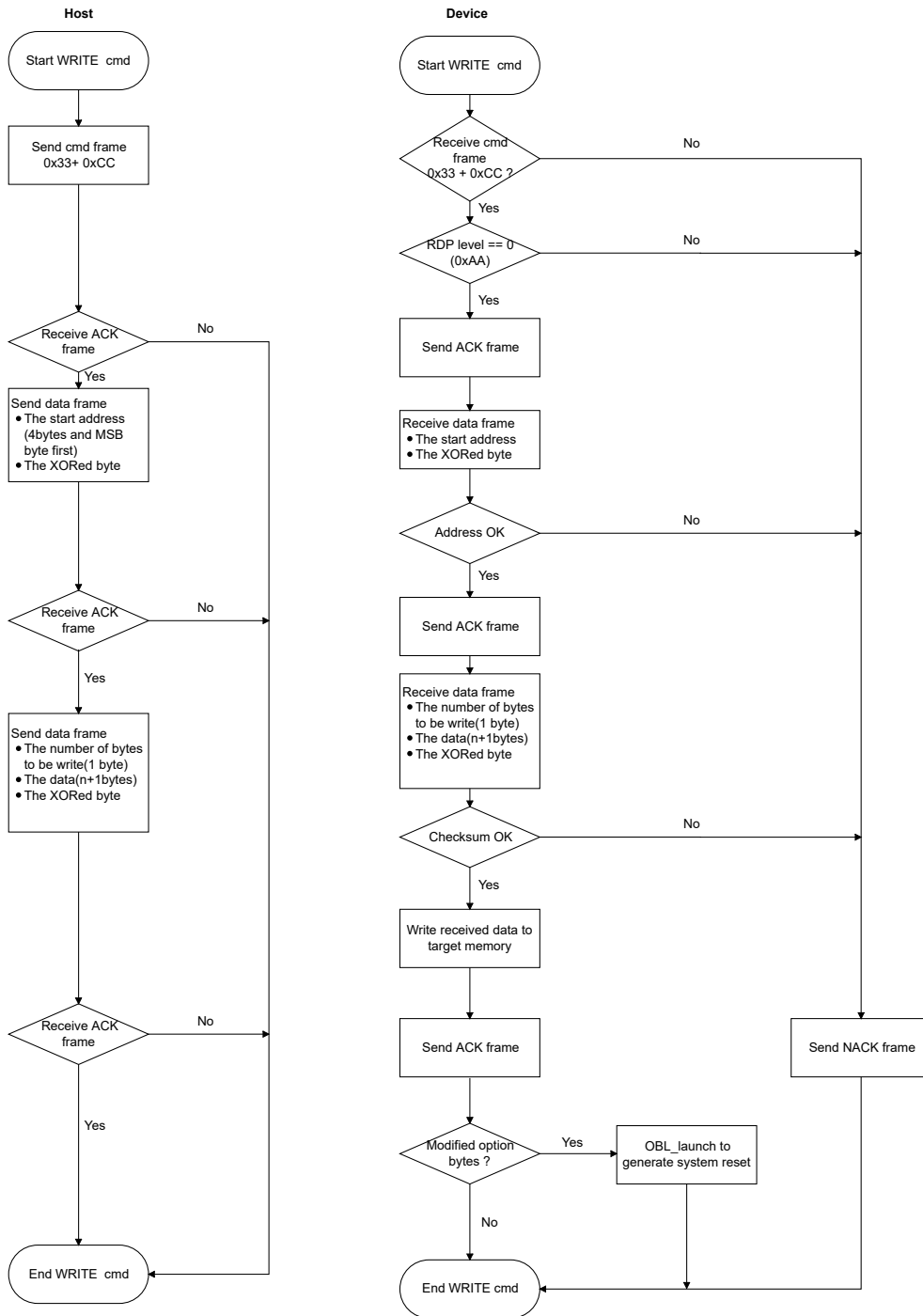
Figure 3-17 IIC Bootloader WRITE Flow Chart
