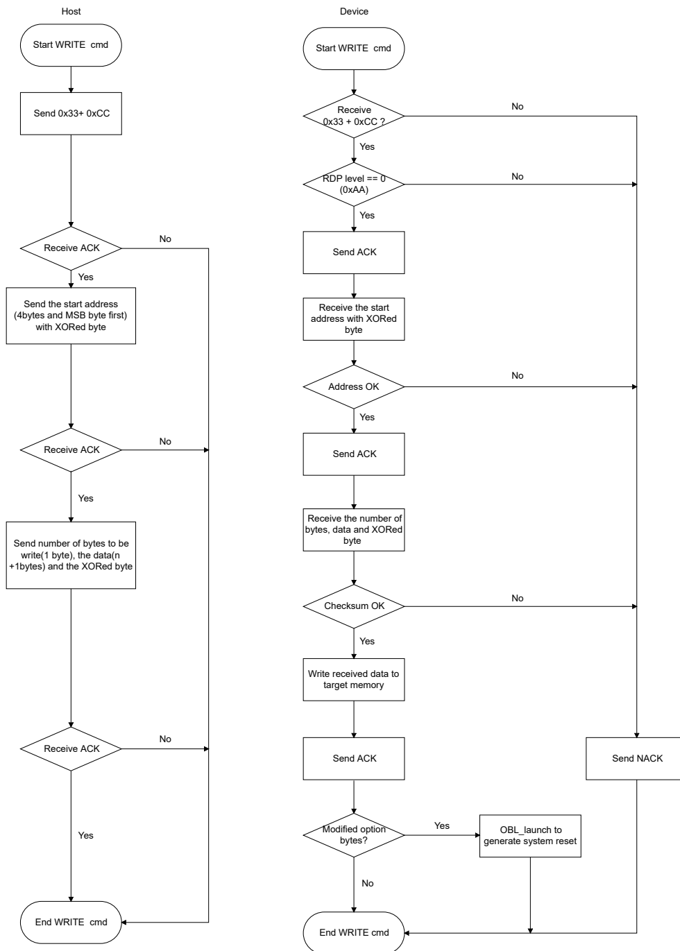
Figure 3-8 USART Bootloader WRITE Flow Chart
