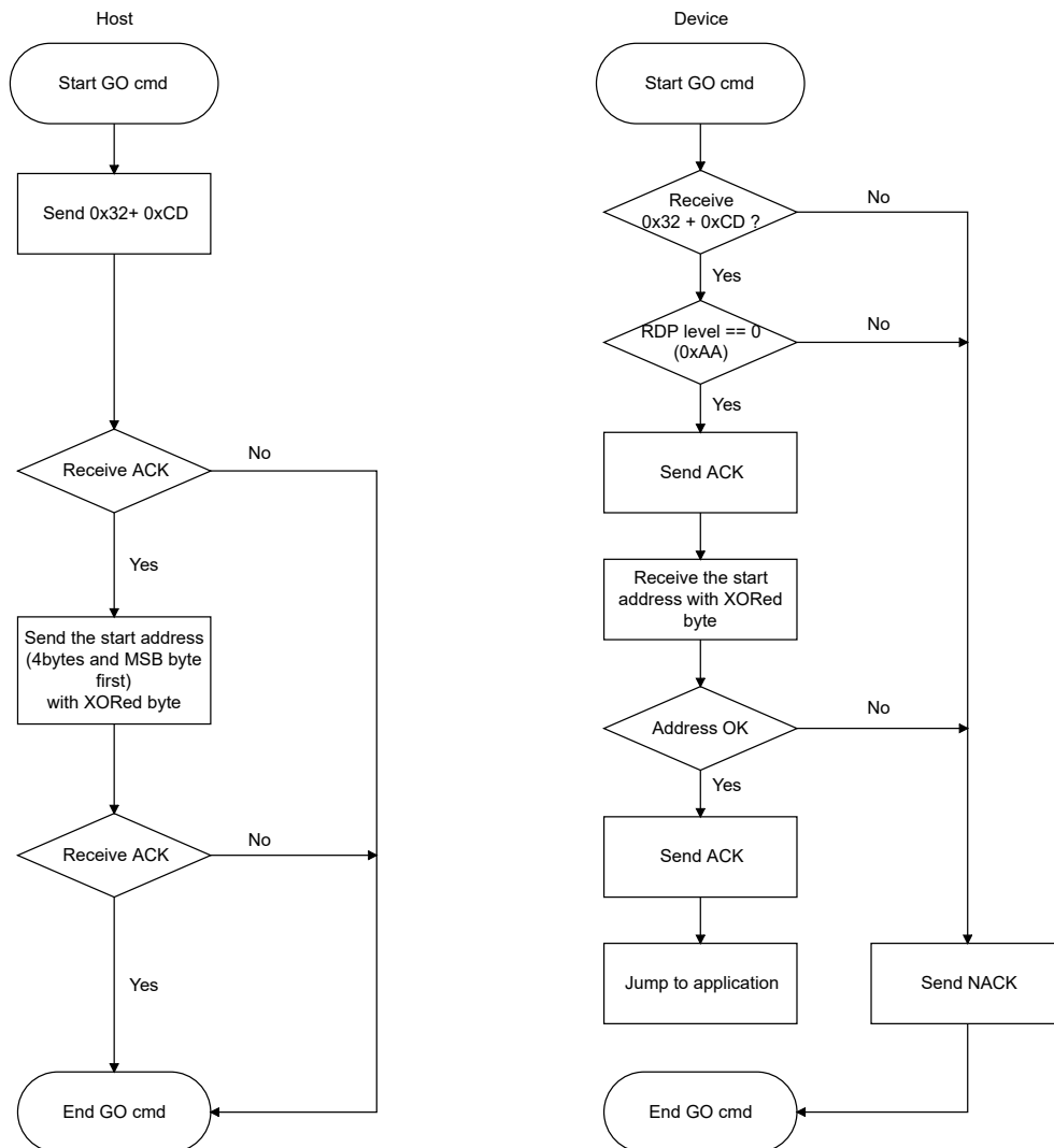
Figure 3-7 USART Bootloader GO Flow Chart
