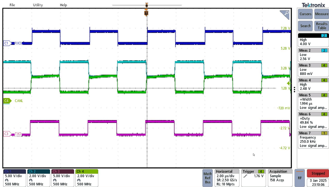
Figure. 4 Waveforms at datarate= 500Kbps, bus load=120Ω, VCCA=3.3V, VCCB=5V
