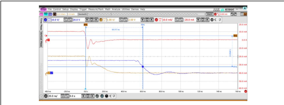
Fig. 8 Propagation Delay Time @ VCC2=15V, 1nF load
