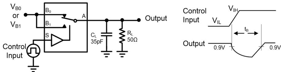
Figure 7. Switch Break Time
