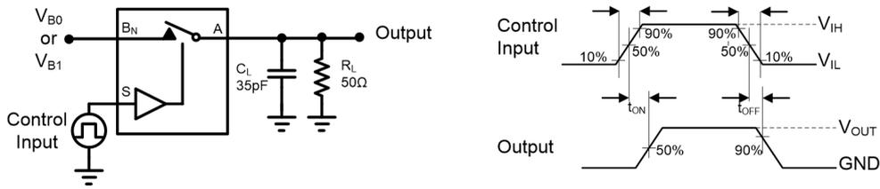
Figure 6. AC Test Circuit and Test Waveforms
