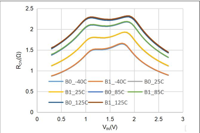
Figure 2.  $R_{ON}$ ,  $V_{CC} = 2.7\text{ V}$ , Temp = -40, 25, 85, 125°C
