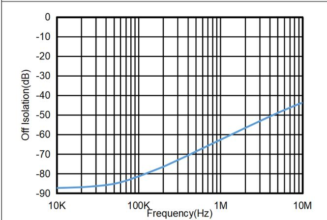
Figure 3. Off-Isolation,  $V_{CC} = 4.5\text{ V}$
