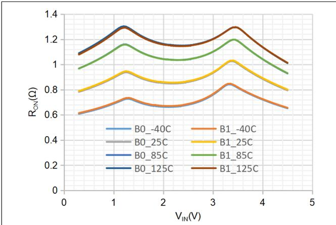
Figure 1.  $R_{ON}$ ,  $V_{CC} = 4.5\text{ V}$ , Temp = -40, 25, 85, 125°C
