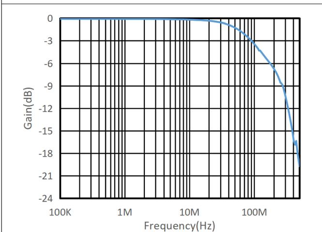
Figure 5. Bandwidth,  $V_{CC} = 4.5\text{ V}$
