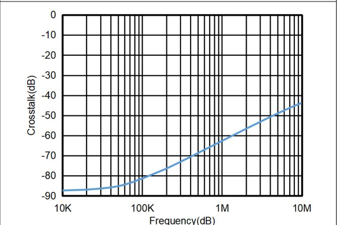
Figure 4. Crosstalk,  $V_{CC} = 4.5\text{ V}$
