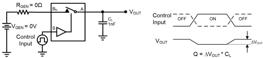
Figure 8. Charge Injection
