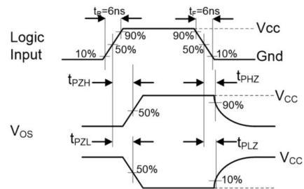
Figure 3. AC Test Circuit and Test Waveforms
