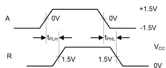
**Figure 5. Receiver Propagation Delay and Data Rate**
