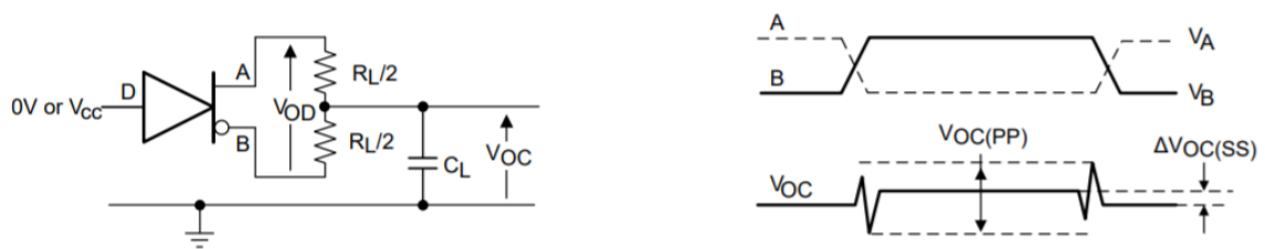
Figure 1. DC Driver Test Circuits
