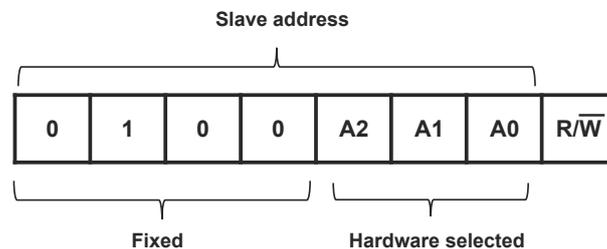
**Figure 8. Slave Device Address**
