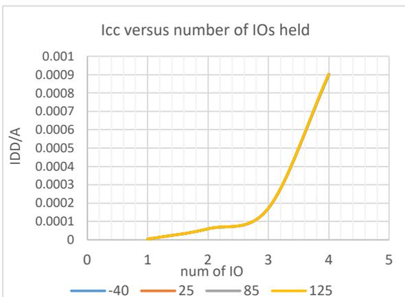
Figure 5. Icc versus Number of I/Os Measurement
