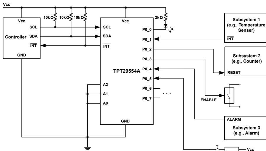
Figure 9. Typical Application Reference Circuit
