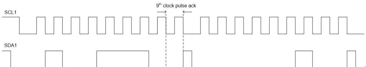
Figure 7. I<sup>2</sup>C BUS (1.65 V ~ 5.5 V) Waveform
