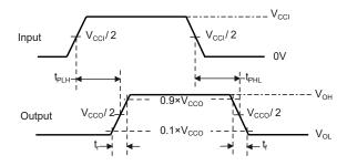
Figure 4. Propagation Delay Times
