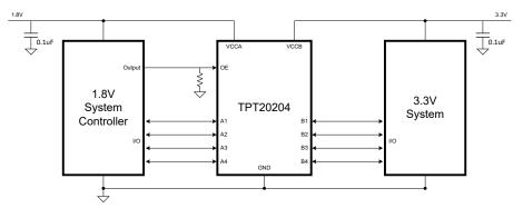
Figure 7. Typical Application Circuit
