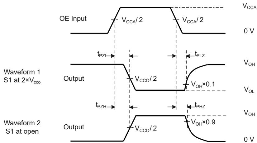
Figure 5. Enable and Disable Times
