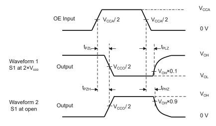
Figure 5. Enable and Disable Times
