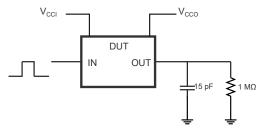
Figure 1. Timing Measurement Load Circuit of Push-Pull Driver
