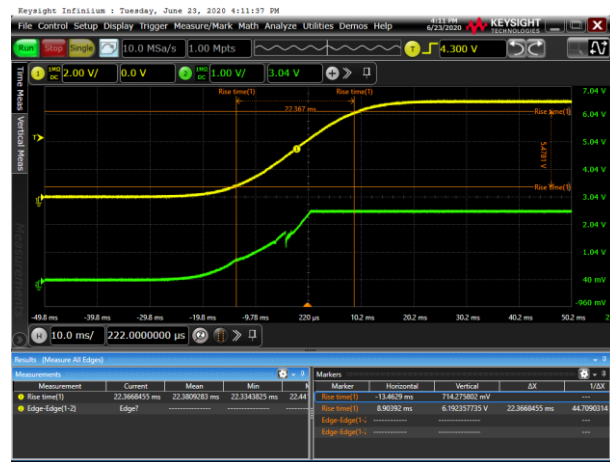
Figure 10. Power Up, 15 ms, V_{BIAS} = 6.5\text{ V} , R_{BIAS} = 20\text{ k}\Omega
