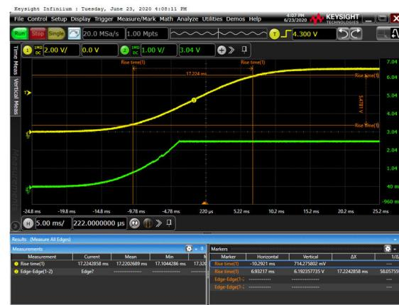
Figure 8. Power up, 15 ms,  $V_{BIAS} = 6.5 \text{ V}$ ,  $R_{BIAS} = 2.5 \text{ k}\Omega$
