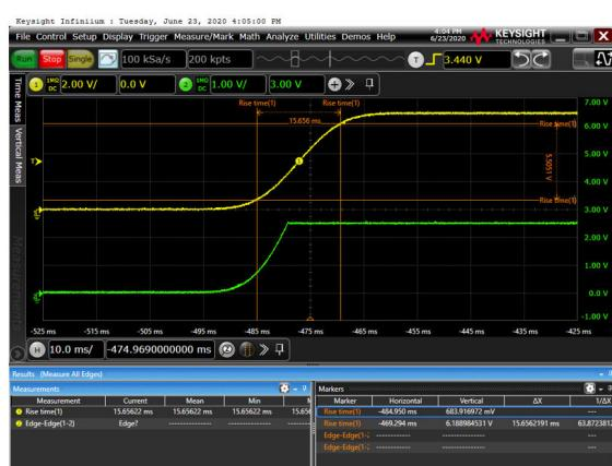
Figure 6. Power Up, 15 ms,  $V_{BIAS} = 6.5$  V,  $R_{BIAS} = 0.5 \text{ k}\Omega$
