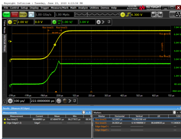
Figure 9. Power Up, 100 \mu\text{s} , V_{BIAS} = 6.5\text{ V} , R_{BIAS} = 20\text{ k}\Omega
