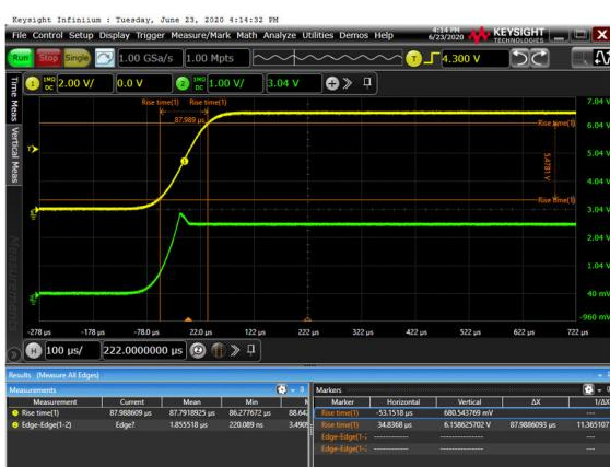
Figure 5. Power Up, 100  $\mu\text{s}$ ,  $V_{BIAS} = 6.5$  V,  $R_{BIAS} = 0.5 \text{ k}\Omega$
