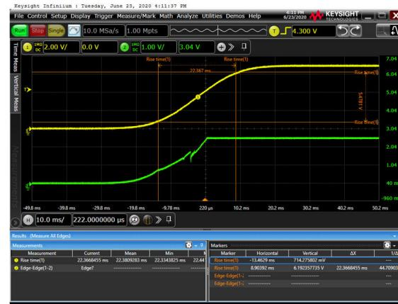
Figure 10. Power up, 15 ms,  $V_{BIAS} = 6.5 \text{ V}$ ,  $R_{BIAS} = 20 \text{ k}\Omega$
