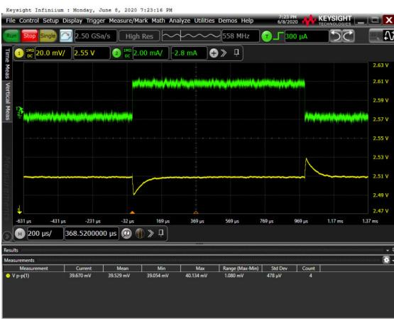
**Figure 13. Load Transient,  $\pm 2$  mA,  $V_{IN} = 5$  V,  $C_{IN} = 1 \mu\text{F}$ ,  $C_{OUT} = 1 \mu\text{F}$ , 20 mV/div**
