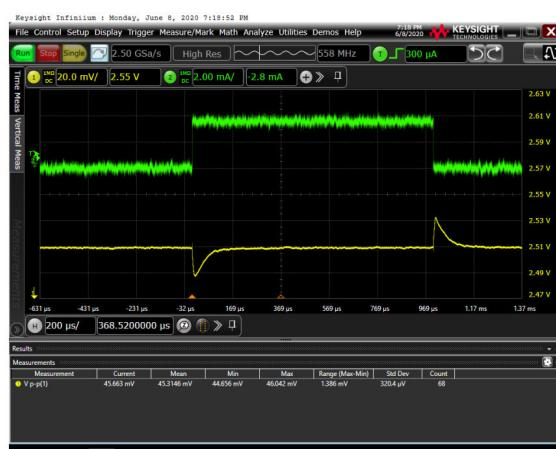
**Figure 14. Load Transient,  $\pm 2$  mA,  $V_{IN} = 2.8$  V,  $C_{IN} = 1 \mu\text{F}$ ,  $C_{OUT} = 1 \mu\text{F}$ , 20 mV/div**
