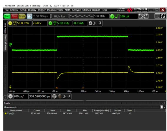
**Figure 11. Load Transient,  $\pm 5$  mA,  $V_{IN} = 5$  V,  $C_{IN} = 1 \mu\text{F}$ ,  $C_{OUT} = 1 \mu\text{F}$ , 50 mV/div**
