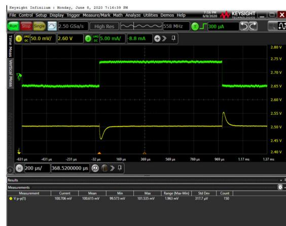
**Figure 12. Load Transient,  $\pm 5$  mA,  $V_{IN} = 2.8$  V,  $C_{IN} = 1 \mu\text{F}$ ,  $C_{OUT} = 1 \mu\text{F}$ , 50 mV/div**
