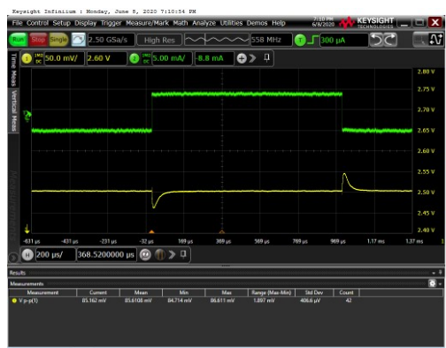
Figure 11. Load Transient, \pm 5\text{ mA} , V_{IN} = 5\text{ V} , C_{IN} = 1\text{ }\mu\text{F} , C_{OUT} = 1\text{ }\mu\text{F} , 50\text{ mV/div}
