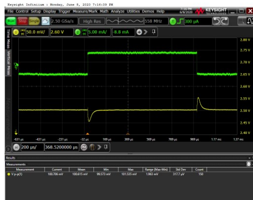
Figure 12. Load Transient, \pm 5\text{ mA} , V_{IN} = 2.8\text{ V} , C_{IN} = 1\text{ }\mu\text{F} , C_{OUT} = 1\text{ }\mu\text{F} , 50\text{ mV/div}
