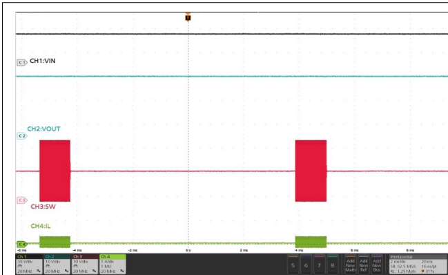
Figure 19. Switching Waveform at 0-A Load Current
