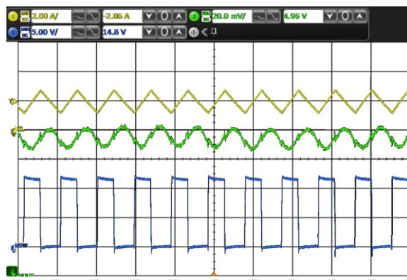
CH1:  $I_{ind}$  CH2:  $V_{OUT}$  CH3: SW
