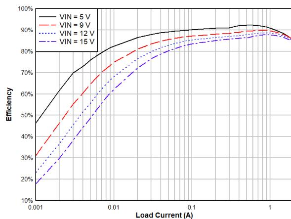
Figure 11. Efficiency vs. Output Current,  $V_{OUT} = 1.8\text{ V}$ ,  $L = 2.2\text{ }\mu\text{H}$
