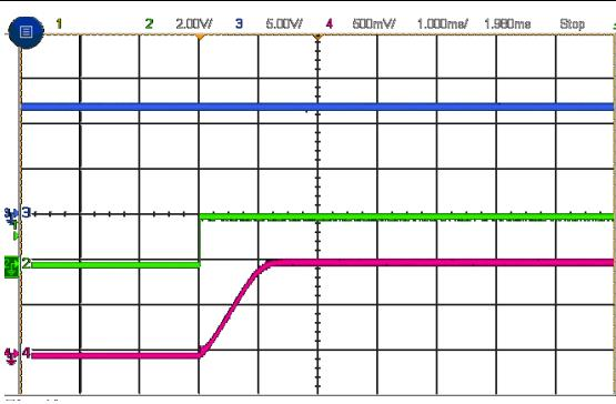
Figure 26. Power-Up Sequence with EN
