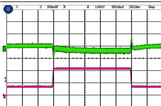
Figure 21. Load Transient
