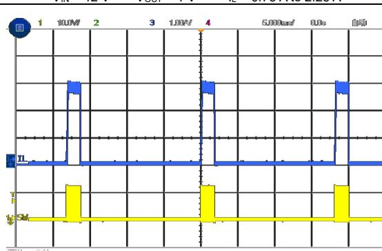
Figure 23. Over-current Hiccup Protection
