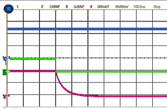
Figure 27. Power-Down Sequence with EN
