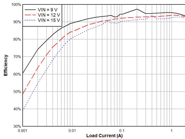
Figure 13. Efficiency vs. Output Current,  $V_{OUT} = 5\text{ V}$ ,  $L = 2.2\text{ }\mu\text{H}$
