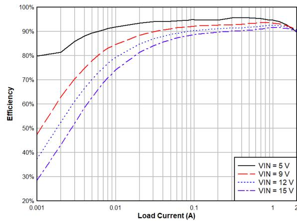
Figure 12. Efficiency vs. Output Current,  $V_{OUT} = 3.3\text{ V}$ ,  $L = 2.2\text{ }\mu\text{H}$
