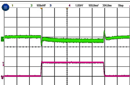
Figure 20. Load Transient
