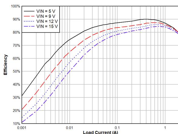
Figure 9. Efficiency vs. Output Current,  $V_{OUT} = 1.05\text{ V}$ ,  $L = 2.2\text{ }\mu\text{H}$
