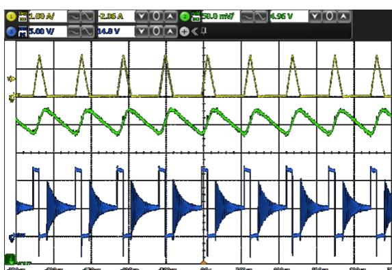
CH1:  $I_{ind}$  CH2:  $V_{OUT}$  CH3: SW
