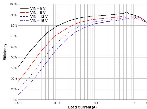
Figure 10. Efficiency vs. Output Current,  $V_{OUT} = 1.5\text{ V}$ ,  $L = 2.2\text{ }\mu\text{H}$
