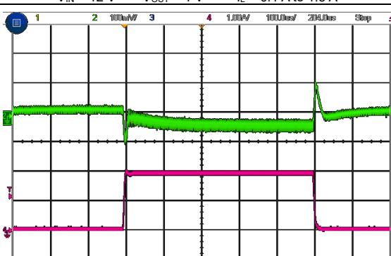
Figure 22. Load Transient
