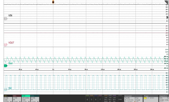
Figure 14. Switching Waveform in CCM Mode
