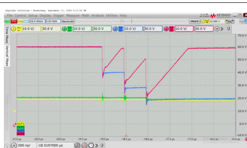
Figure 15. Discharge During Charging
