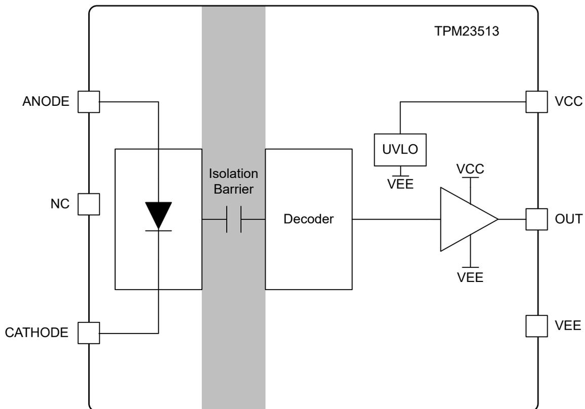
Figure 10. Functional Block Diagram
