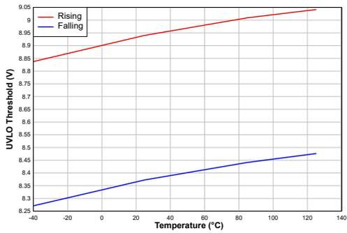
Figure 7. UVLO Threshold vs. Temperature
