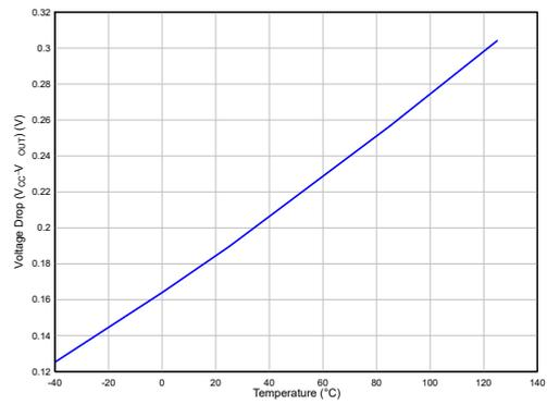
Figure 4. VOH Voltage Drop vs. Temperature
