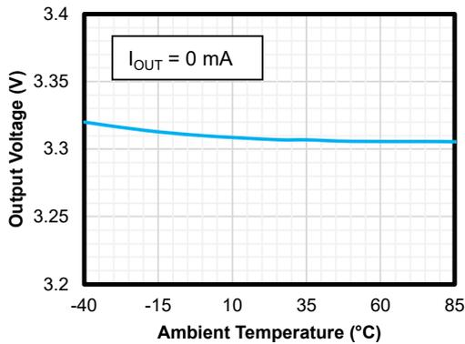
Figure 5. Output Accuracy vs. Ambient Temperature
