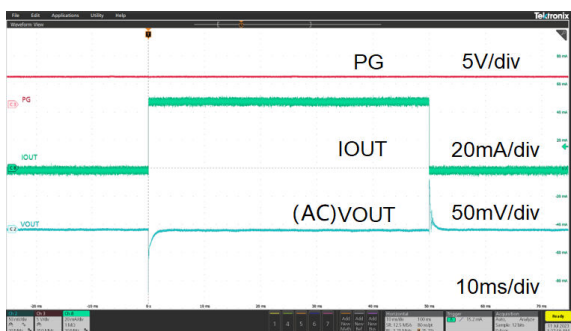
V_{IN} = 13.5 \text{ V} , V_{OUT} = 5 \text{ V} , C_{OUT} = 10 \mu\text{F} , I_{OUT} = 1 \text{ mA to } 50 \text{ mA}
