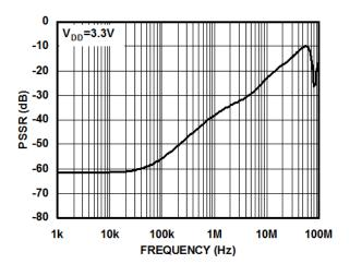
Figure9. PSRR Vs. Frequency
