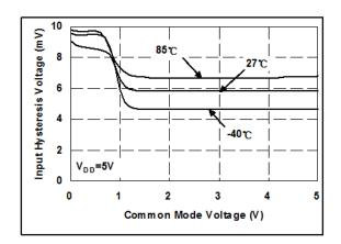
Input Hysteresis Voltage V.S. Common Mode Voltage
