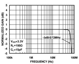
Figure4. Large-Scale Frequency Response
