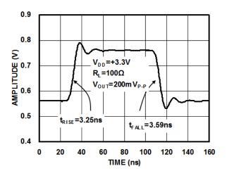
Figure12. Small-Signal Pulse Response Vs. Time
