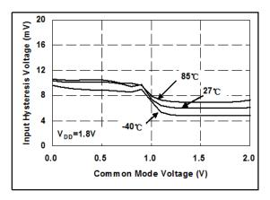
Input Hysteresis Voltage V.S. Common Mode Voltage
