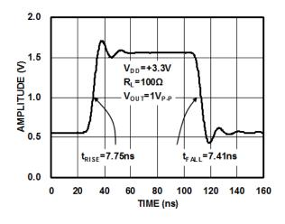
Figure11. Large-Signal Pulse Response Vs. Time
