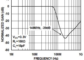
Figure8. Stop Band Attenuation
