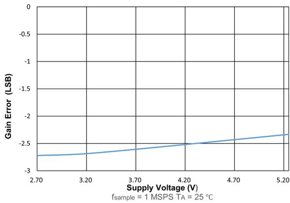
Figure 10. Gain Error vs. Supply Voltage (V (+VA))
