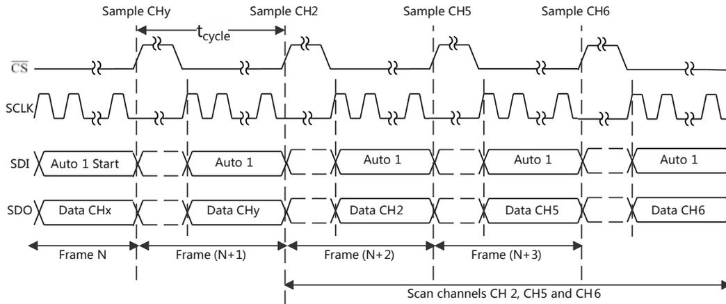
Figure 22. Example Auto-1 Mode Timing Diagram
