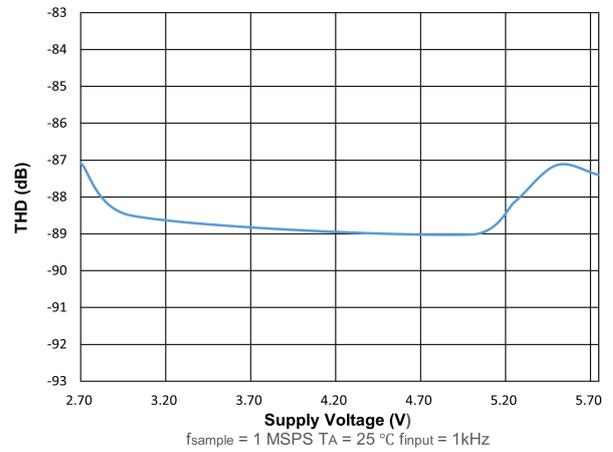
Figure 15. THD vs. Supply Voltage (V (+VA))
