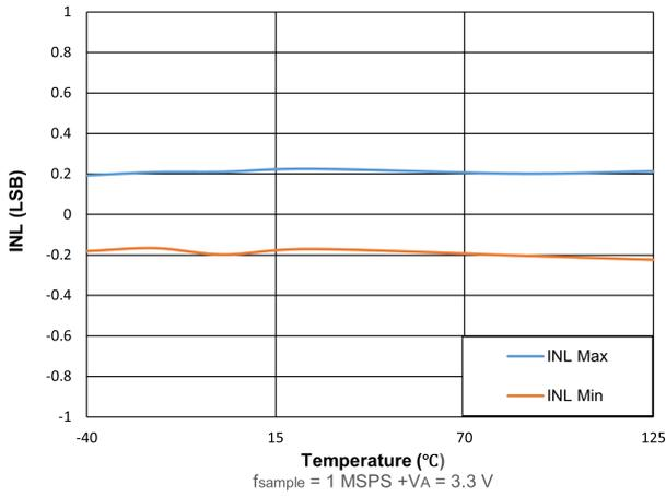
Figure 8. INL vs. Temperature
