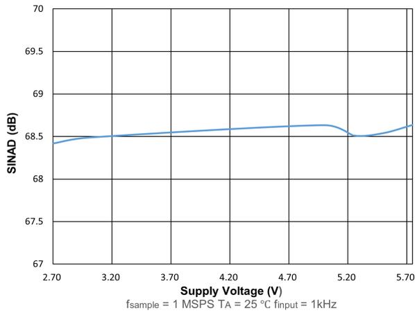
Figure 14. SINAD vs. Supply Voltage (V (+VA))
