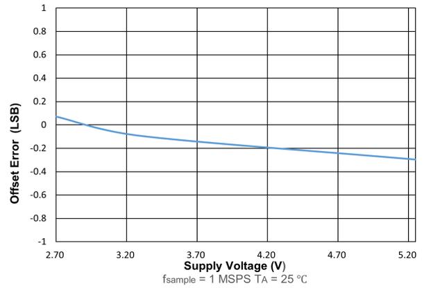
Figure 9. Offset Error vs. Supply Voltage (V (+VA))
