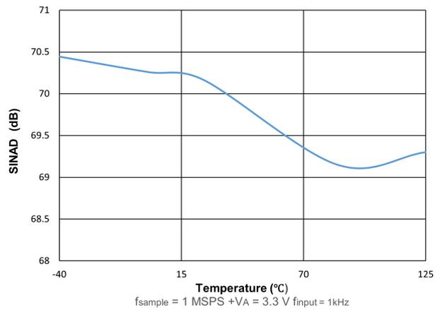
Figure 17. SINAD vs. Temperature
