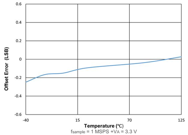
Figure 11. Offset Error vs. Temperature
