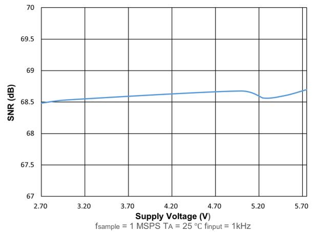
Figure 13. SNR vs. Supply Voltage (V (+VA))
