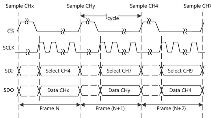
Figure 21. Example Manual Mode Timing Diagram
