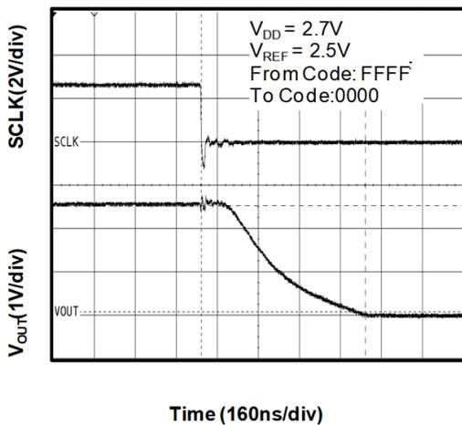
Figure 17. Full-Scale Settling Time (2.7-V Falling Edge)
