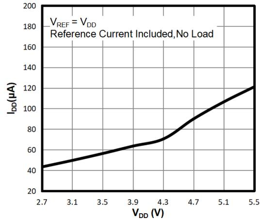
Figure 16. Supply Current vs. Supply Voltage (TPC116S8)
