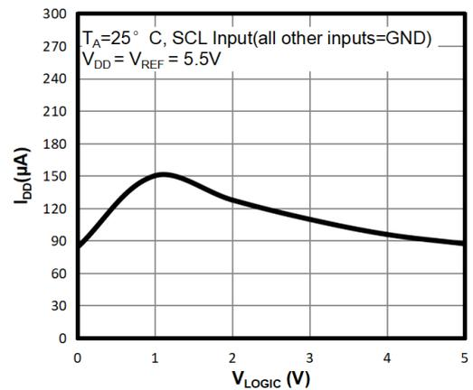
Figure 14. Supply Current vs. Logic Input Voltage (TPC116S8)
