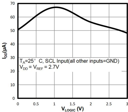
Figure 15. Supply Current vs. Logic Input Voltage (TPC116S8)
