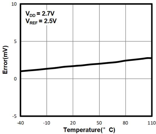
Figure 11. Full-Scale Error vs. Temperature (TPC116S8)
