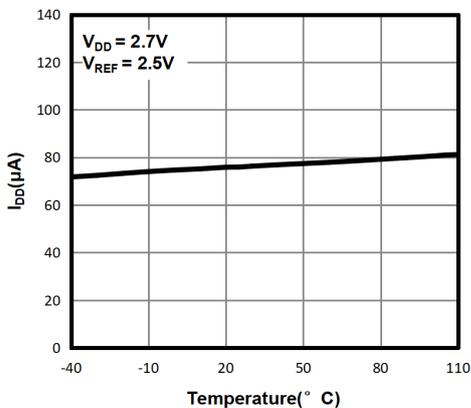
Figure 7. Power-Supply Current vs. Temperature (TPC116S8)
