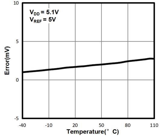
Figure 10. Full-Scale Error vs. Temperature (TPC116S8)
