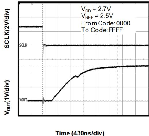
Figure 20. Full-Scale Settling Time (2.7-V Rising Edge)
