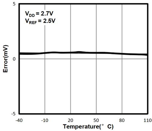
Figure 9. Zero-Scale Error vs. Temperature (TPC116S8)
