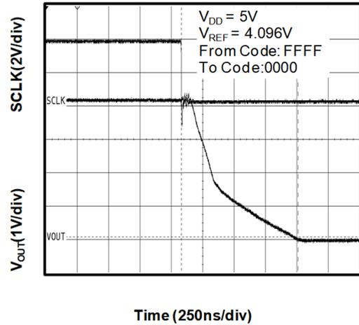
Figure 18. Full-Scale Settling Time (5-V Falling Edge)
