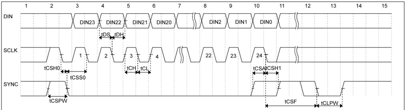
Figure 2. 24-Bit Serial-Interface Timing Diagram (TPC116S8)
