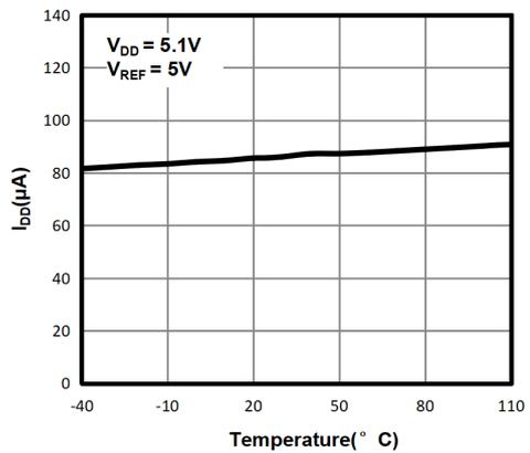
Figure 6. Power-Supply Current vs. Temperature (TPC116S8)
