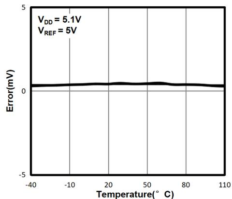
Figure 8. Zero-Scale Error vs. Temperature (TPC116S8)
