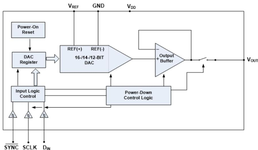
Figure 21. Block Diagram of One DAC
