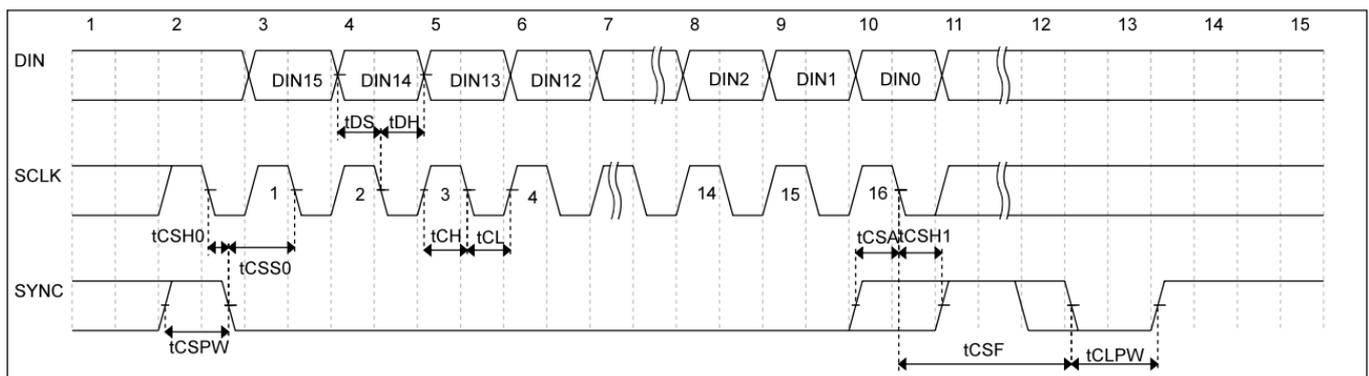
Figure 1. 16-Bit Serial-Interface Timing Diagram (TPC112S8)
