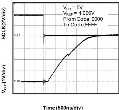
Figure 19. Full-Scale Settling Time (5-V Rising Edge)
