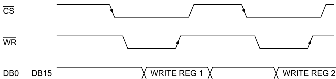
Figure 27. Parallel Interface Register Write
