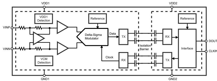
**Figure 15. Functional Block Diagram**
