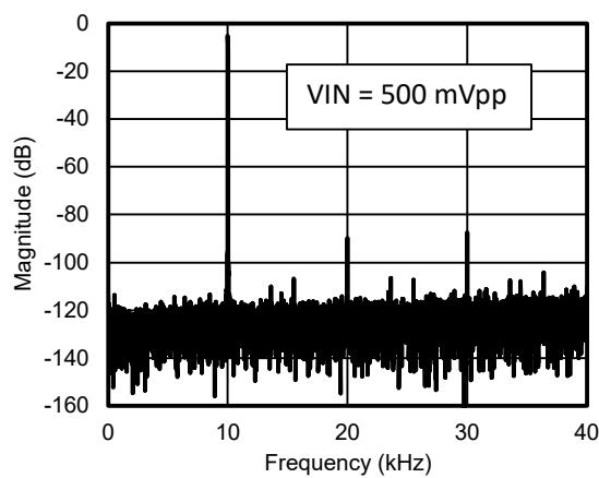
**Figure 14. Frequency Spectrum with 10-kHz Input Signal**
