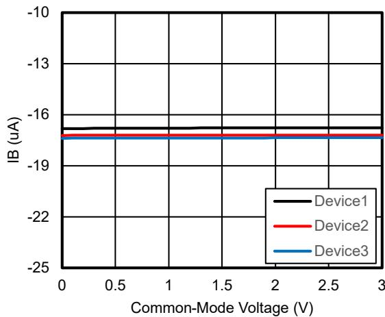
**Figure 7.  $I_B$  vs. Common-Mode Voltage**
