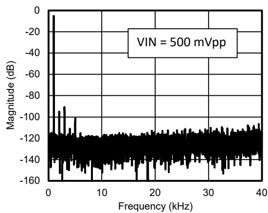
**Figure 13. Frequency Spectrum with 1-kHz Input Signal**
