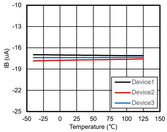
**Figure 8.  $I_B$  vs. Temperature**
