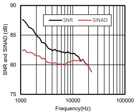
**Figure 12. SNR and SINAD vs. Input Signal Frequency**
