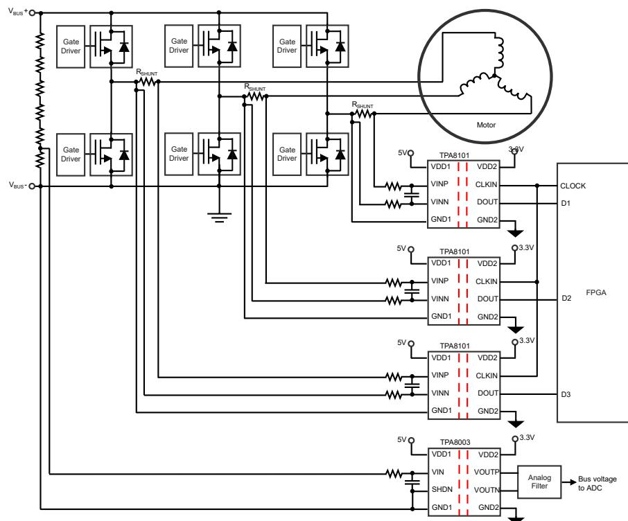
Figure 16. Application Schematic
