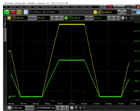
G = 1, V_{IN} = 1/2 V_S during Power On and Off Yellow: + V_S ; Green: Output
