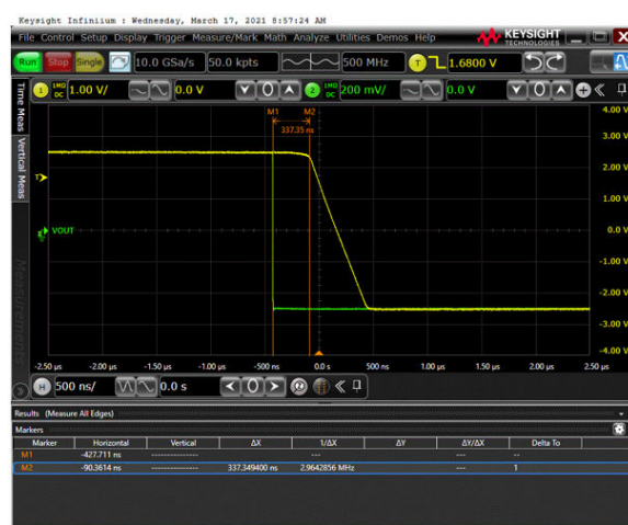
Figure 16. Overload Recovery at Positive Rail
