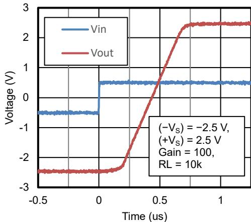
**Figure 12. Overload Recovery at Positive Rail**
