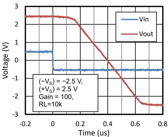
**Figure 11. Overload Recovery at Negative Rail**
