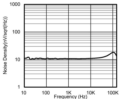
**Figure 3. Voltage Noise Spectral Density vs. Frequency**
