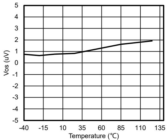
**Figure 8. V<sub>os</sub> vs. Temperature**
