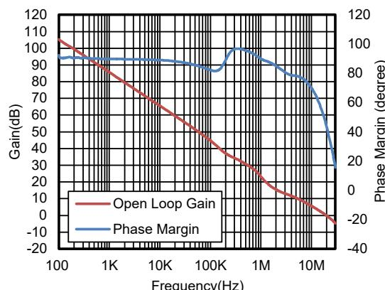
**Figure 4. Open-Loop Gain and Phase Margin vs. Frequency,  $R_L = 10$  k $\Omega$**
