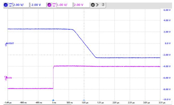
Figure 14. Overload Recovery at Negative Rail
