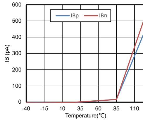
**Figure 10.** I<sub>B</sub> vs. Temperature, V<sub>s</sub> = 16 V, V<sub>cm</sub> = 8 V
