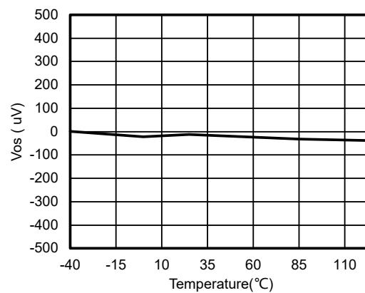
**Figure 8.** V<sub>os</sub> vs. Temperature
