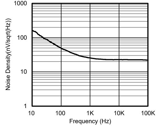
**Figure 18. Voltage Noise Spectral Density vs. Frequency**
