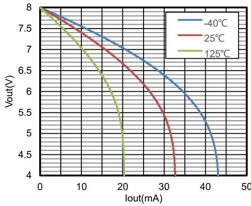
**Figure 11.** Output Voltage vs. Output Current, Source, (-V<sub>s</sub>) = -8 V, (+V<sub>s</sub>) = 8 V
