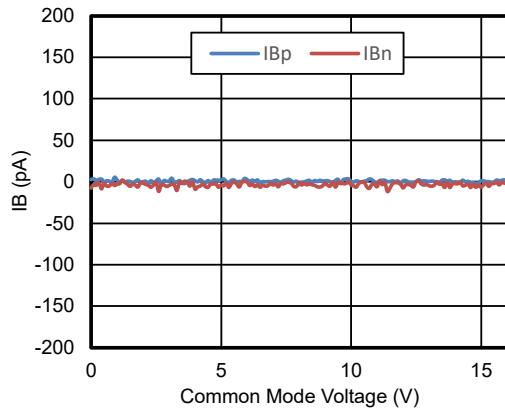
**Figure 9.** I<sub>B</sub> vs. Common Voltage, V<sub>s</sub> = 16 V
