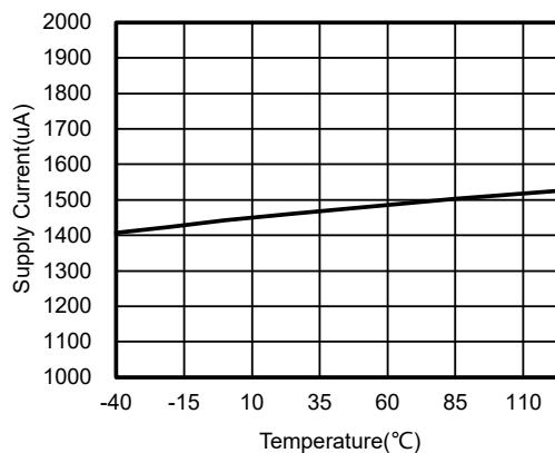
**Figure 2. Supply Current vs. Temperature, TPA3662**
