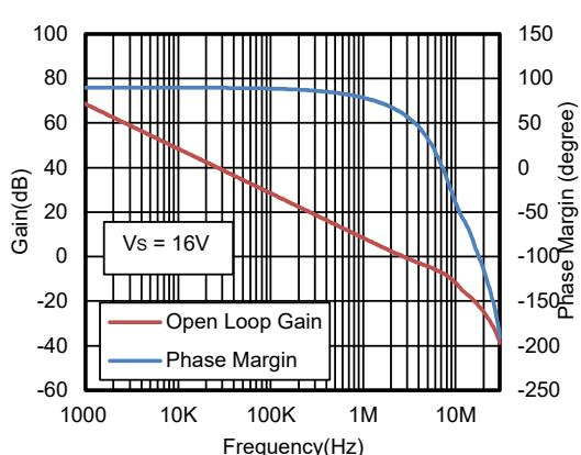
**Figure 6. Open-Loop Gain and Phase Margin vs. Frequency,  $R_L = 10$  kΩ,  $C_L = 100$  pF**
