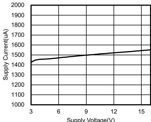
**Figure 1. Supply Current vs. Supply Voltage, TPA3662**
