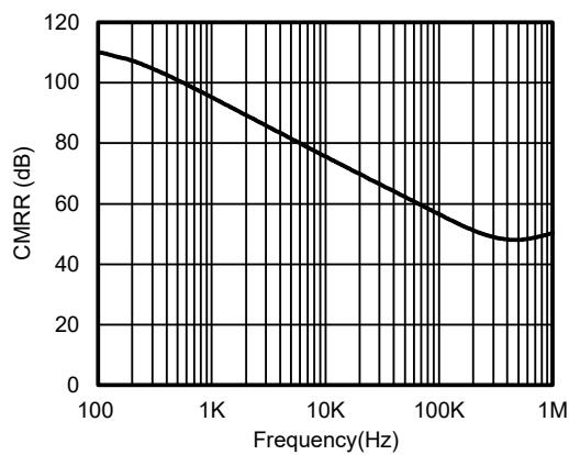
**Figure 5. CMRR vs. Frequency, Vs = 16V**
