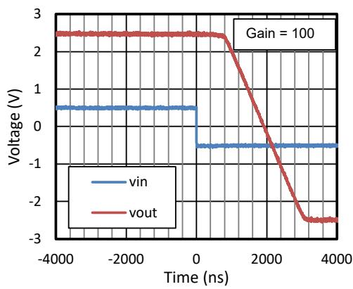
**Figure 14. Overload Recovery at Positive Rail**
