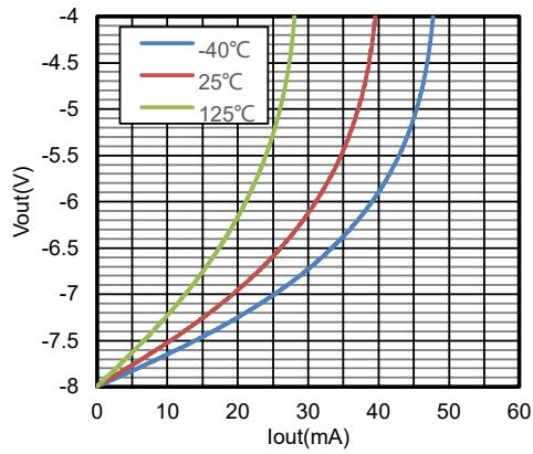
**Figure 12.** Output Voltage vs. Output Current, Sink, (-V<sub>s</sub>) = -8 V, (+V<sub>s</sub>) = 8 V
