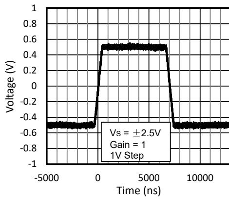
**Figure 16. 1-V Large-Signal Step Response**
