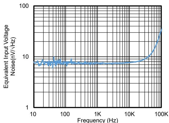
**Figure 13. Voltage Noise Spectral Density vs. Frequency**
