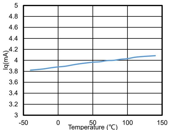
**Figure 4.  $I_Q$  vs. Temperature, 30-V Supply, TPA1882**
