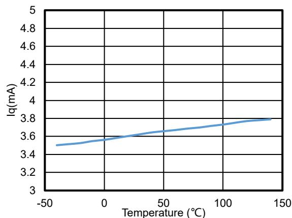
**Figure 3.  $I_Q$  vs. Temperature, 5-V Supply, TPA1882**
