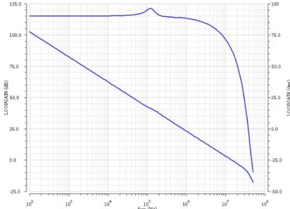
**Figure 6. Open Loop Gain and Phase vs. Frequency**
