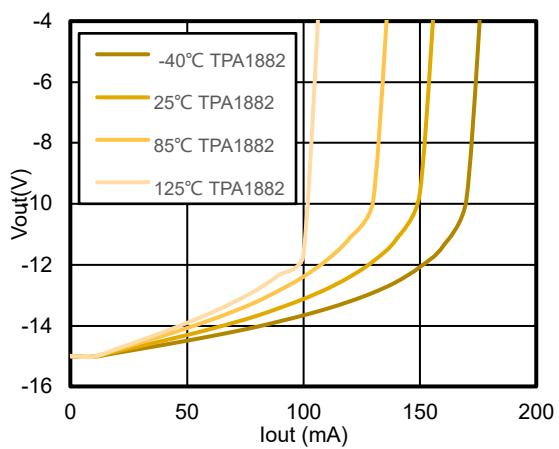
**Figure 16. V<sub>OUT</sub> vs. I<sub>OUT</sub>, Sink**
