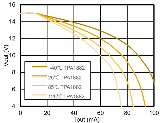
**Figure 15. V<sub>OUT</sub> vs. I<sub>OUT</sub>, Source**
