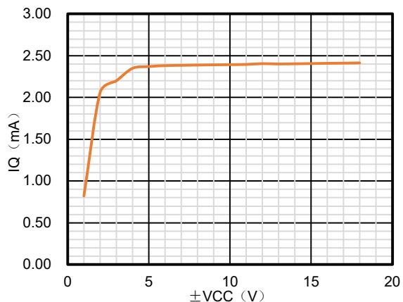
**Figure 2. I<sub>Q</sub> vs. Supply Voltage**
