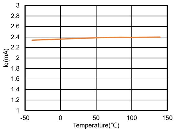
**Figure 4. I<sub>Q</sub> vs. Temperature, ±15-V Supply, TPA1862**
