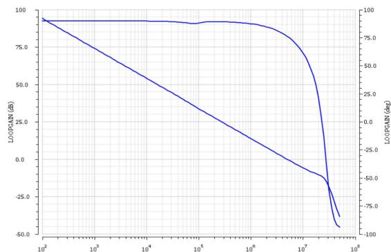
**Figure 6. Open-Loop Gain and Phase vs. Frequency,  $R_L = 10$  k $\Omega$ ,  $C_L = 50$  pF**
