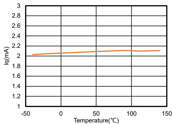
**Figure 3. I<sub>Q</sub> vs. Temperature, ±2.5-V Supply, TPA1862**
