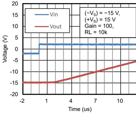
Figure 13. Overload Recovery at Negative Rail
