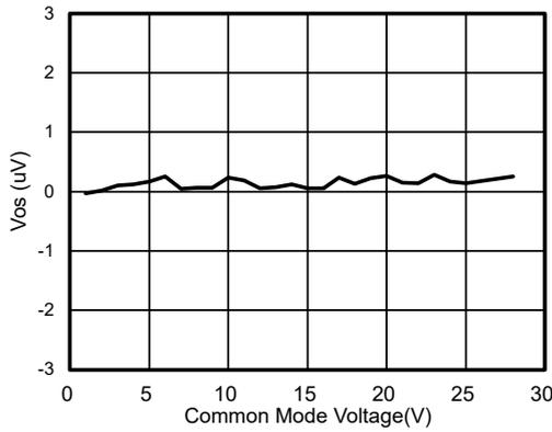
Figure 9.  $V_{OS}$  vs  $V_{CM}$ ,  $V_S = 30\text{ V}$
