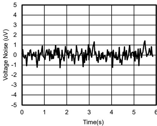
Figure 3. 0.1 to 10 Hz Voltage Noise
