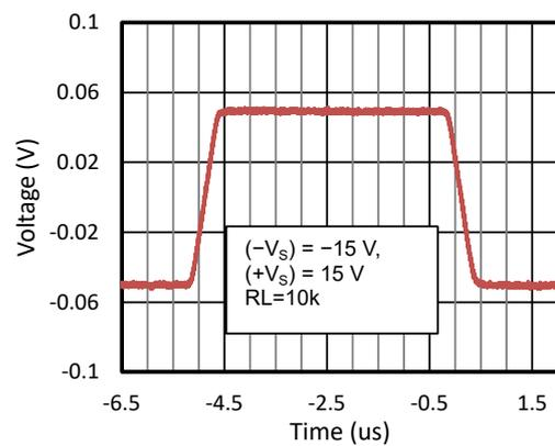
Figure 12. Small Signal Step Response
