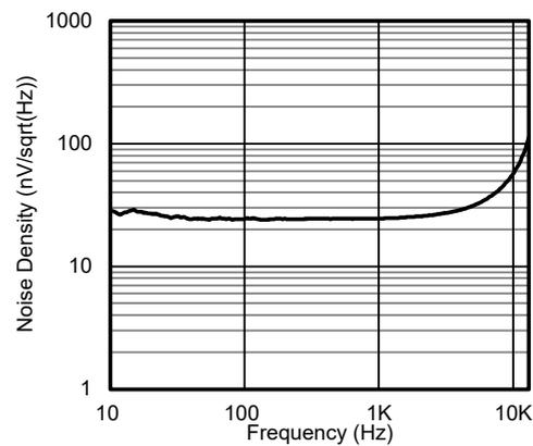
Figure 4. Voltage Noise Spectral Density vs Frequency
