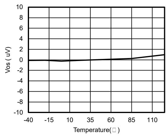
**Figure 10.  $V_{OS}$  vs. Temperature**
