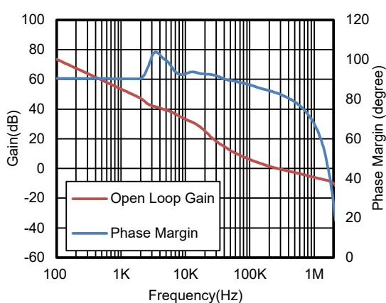
**Figure 6. Open-Loop Gain and Phase Margin vs. Frequency,  $R_L = 10$  k $\Omega$**
