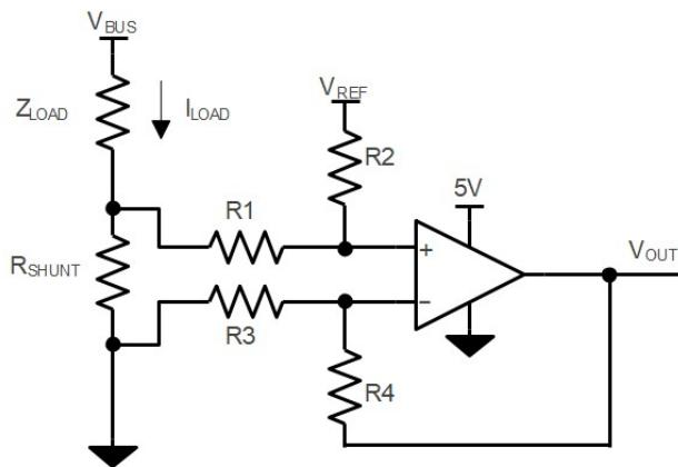
$$V_{OUT} = (I_{LOAD} \times R_{SHUNT}) \times (R_2 / R_1) + V_{REF}$$
