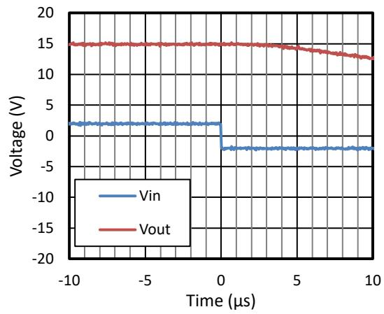
**Figure 12. Overload Recovery at Positive Rail**
