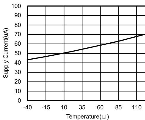
**Figure 2. Supply Current vs. Temperature**
