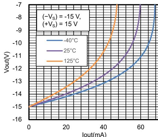
**Figure 14. Output Voltage vs. Output Current, Sink, ( $-V_S$ )
