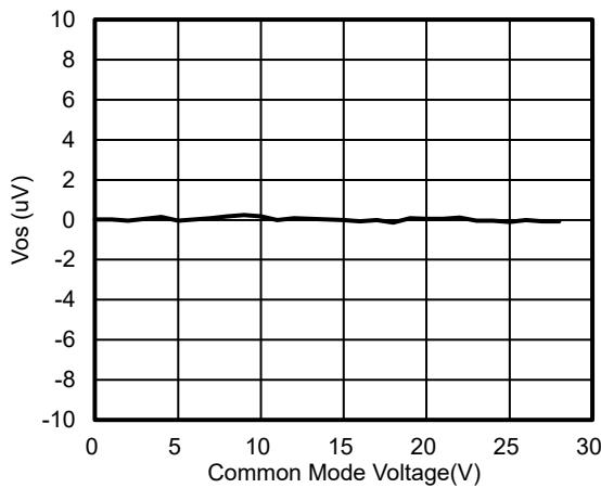
**Figure 9.  $V_{OS}$  vs.  $V_{CM}$ ,  $V_S = 30$  V**
