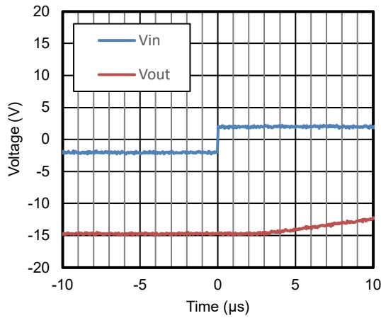
**Figure 11. Overload Recovery at Negative Rail**
