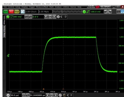
Voltage: 500 mV/div for Output, Time: 50 us/div G=10, VREF = GND; VIN=2 mVPP, Load R=10 K C=100 pF
