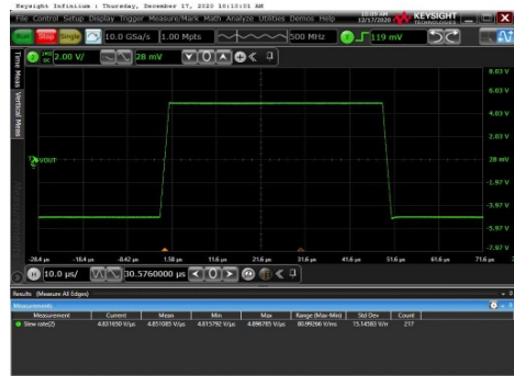
Voltage: 2 V/div for Output, Time: 10 us/div G = 1, V REF = GND; V IN = 10V PP , Load R = 10 K
