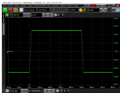
Voltage: 2 V/div for Output, Time: 10 us/div G = 1, V REF = GND; V IN = 10V PP , Load R = 10 K, C = 100 pF
