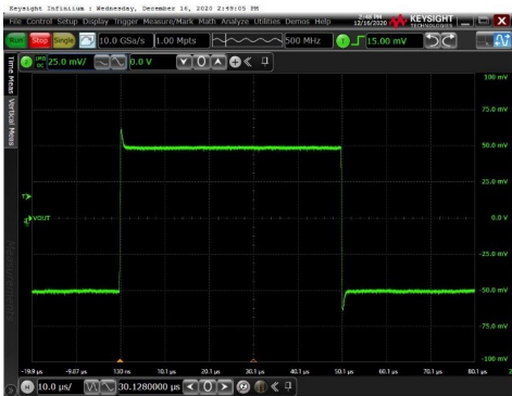
Voltage: 25 mV/div for Output, Time: 10 us/div G=1, VREF = GND; VIN=100 mVPP, Load R=10 K C=100 pF
