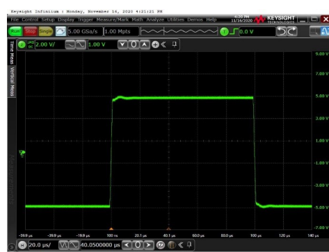
Voltage: 2 V/div for Output, Time: 20 us/div G = 10, V REF = GND; V IN = 1V PP , Load R = 10 K, C = 100 pF
