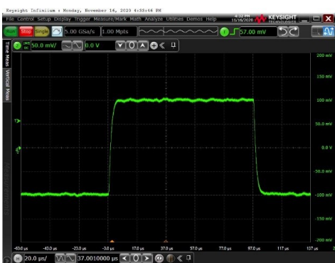
Voltage: 50 mV/div for Output, Time: 20 us/div G=100, VREF = GND; VIN=2 mVPP, Load R=10 K C=100 pF
