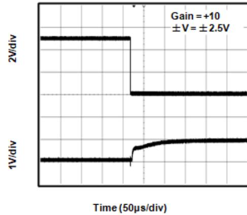
Figure 16. Positive Over-Voltage Recovery
