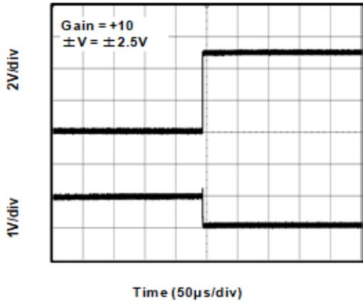
Figure 15. Negative Over-Voltage Recovery
