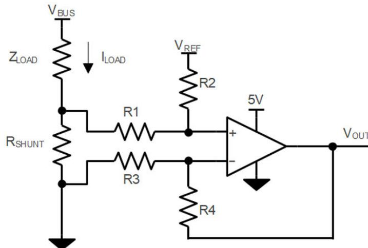
$$V_{OUT} = (I_{LOAD} \times R_{SHUNT}) \times (R_2 / R_1) + V_{REF}$$
