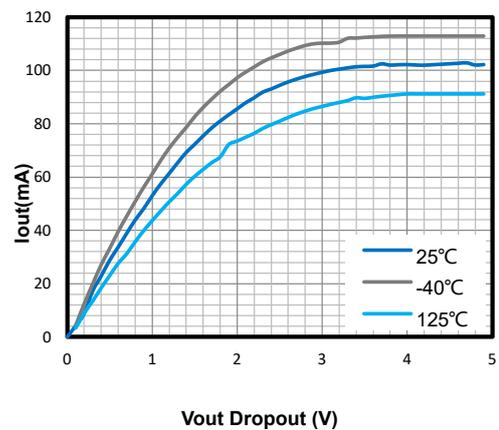
Figure 18. Positive Output Swing vs. Load Current
