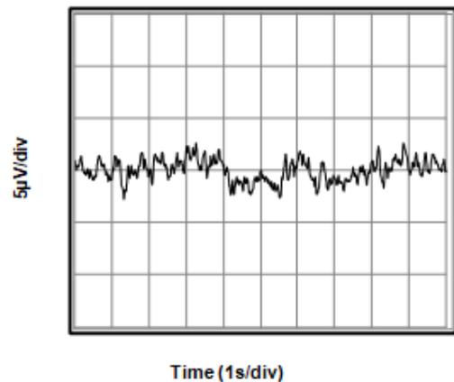
Figure 12. 0.1-Hz to 10-Hz Input Voltage Noise
