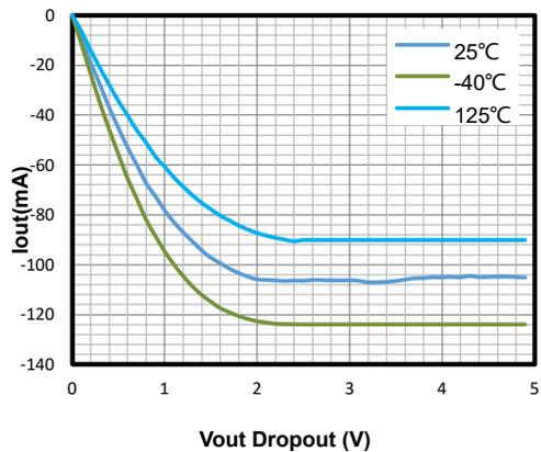
Figure 17. Negative Output Swing vs. Load Current
