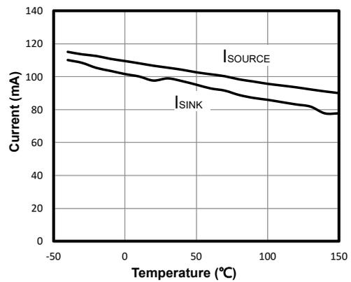
Figure 4. Short Circuit Current vs. Temperature
