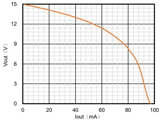
**Figure 15. V<sub>OUT</sub> vs. I<sub>OUT</sub>, Source**
