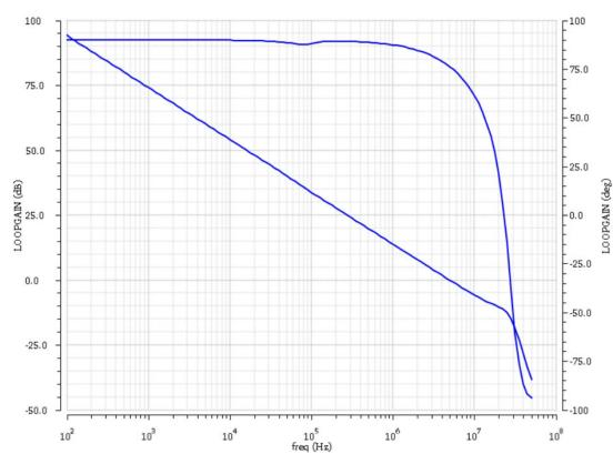
**Figure 6. Open-Loop Gain and Phase vs. Frequency**
