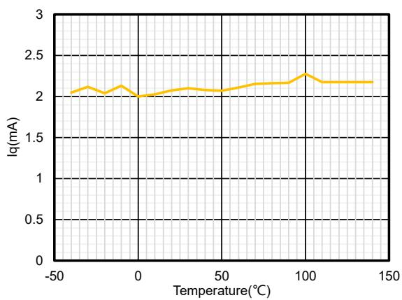
**Figure 3.  $I_Q$  vs. Temperature,  $\pm 2.5$ -V Supply**
