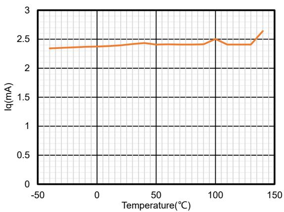
**Figure 4.  $I_Q$  vs. Temperature,  $\pm 15$ -V Supply**
