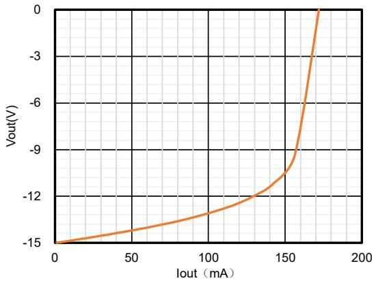
**Figure 16. V<sub>OUT</sub> vs. I<sub>OUT</sub>, Sink**
