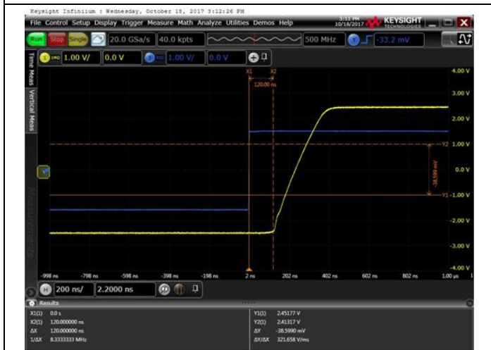
Voltage: 1 V/div, Time: 200 ns/div V_s = 5V , V_{IN} = 2V , R_L = \text{Open} , G = 3 Figure 23. Positive Overload Recovery
