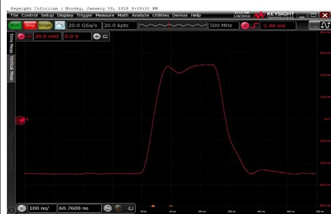
Voltage: 20 mV/div, Time: 100 ns/div V_S = \pm 15V , R_L = 2K , C_L = 100\text{ pF} , G=1 Figure 25. 100-mV Signal Step Response
