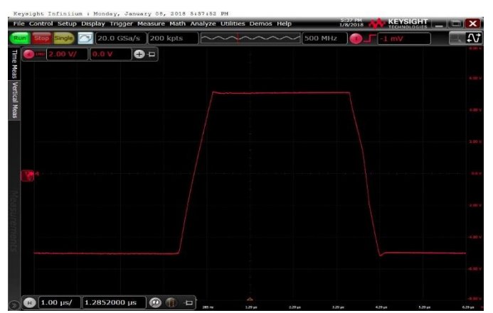
Voltage: 2 V/div, Time: 1 \mu s/div V_S = \pm 15V , R_L = 2K , C_L = 100\text{ pF} , G=1 Figure 26. 10-V Signal Step Response
