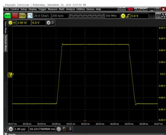
Voltage: 5 V/div, Time: 1  $\mu$ s/div $R_L = 2 \text{ k}\Omega$ ,  $C_L = 100 \text{ pF}$ ,  $G = 1$
