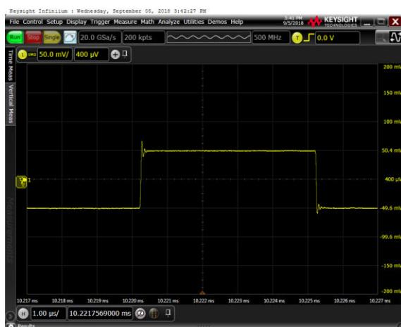
Voltage: 50 mV/div, Time: 1  $\mu$ s/div $R_L = 2 \text{ k}\Omega$ ,  $C_L = 100 \text{ pF}$ ,  $G = 1$
