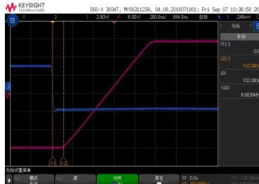
**Figure 16. Negative Overload Recovery**
