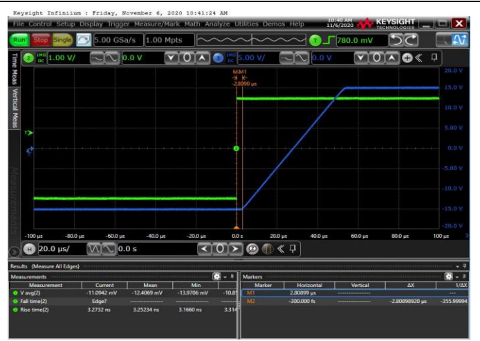
Voltage: 5V/div for Output, Time: 10 \mu s/div G=10, VREF = GND; VIN=5VPP Figure 14. Negative Overload Recovery
