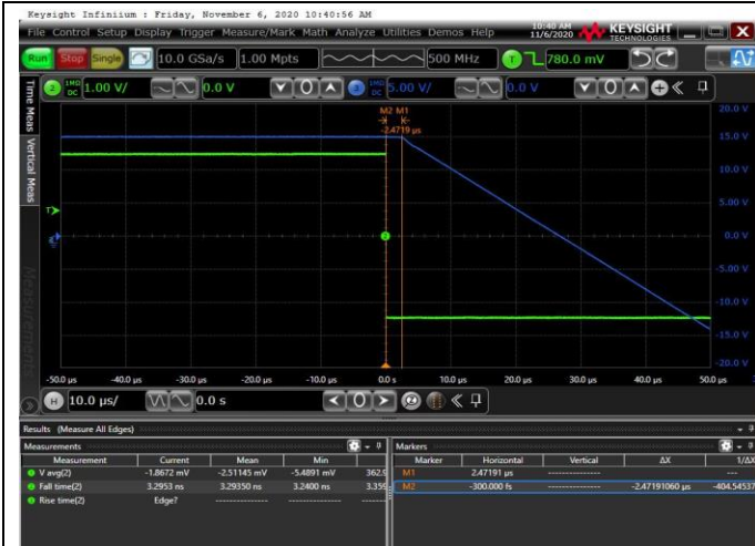
Voltage: 5V/div for Output, Time: 10 \mu s/div G=10, VREF = GND; VIN=5VPP Figure 13. Positive Overload Recovery
