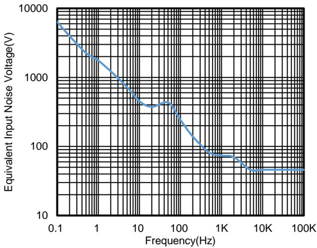
Figure 9. Voltage Noise Spectral Density vs. Frequency
