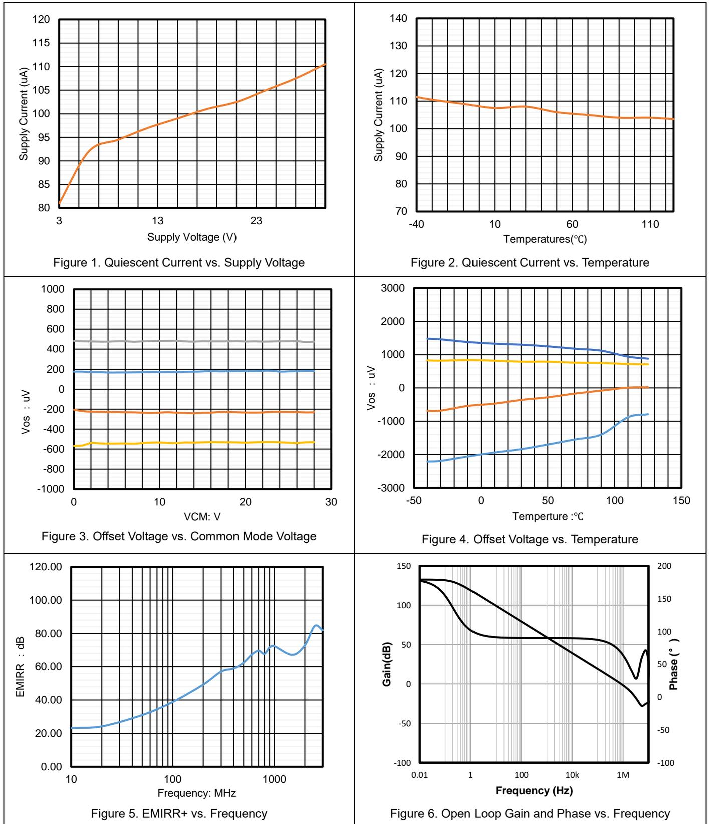
All test conditions:  $V_S = \pm 15\text{ V}$ ,  $V_{CM} = 0\text{ V}$ ,  $R_L = 10\text{ k}\Omega$ , unless otherwise specified.
